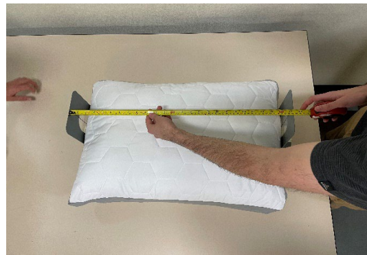
Figure 2: Length Measurement of Pillow with 90° Straightedges – Loose Fill Pillows
