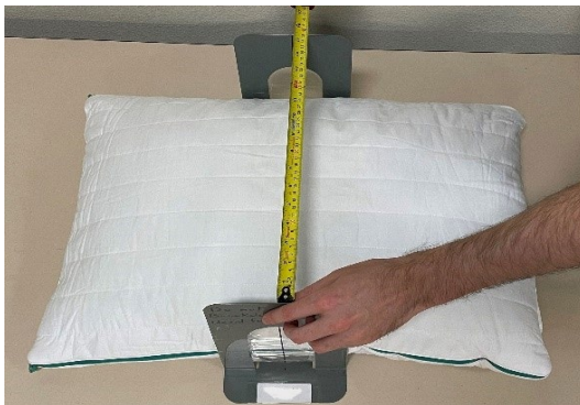
Figure 6: Width Measurement of Pillow with 90° Straightedges – Foam Pillows
