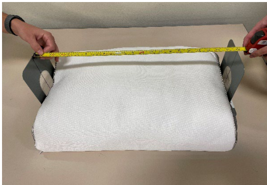
Figure 3: Length Measurement of Pillow with 90° Straightedges – Foam Pillow
