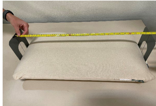
Figure 3: Length Measurement of Pillow with 90° Straightedges – Foam Pillow
