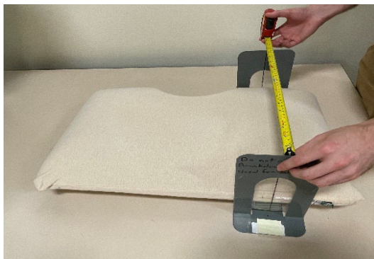
Figure 6: Width Measurement of Pillow with 90° Straightedges – Foam Pillows
