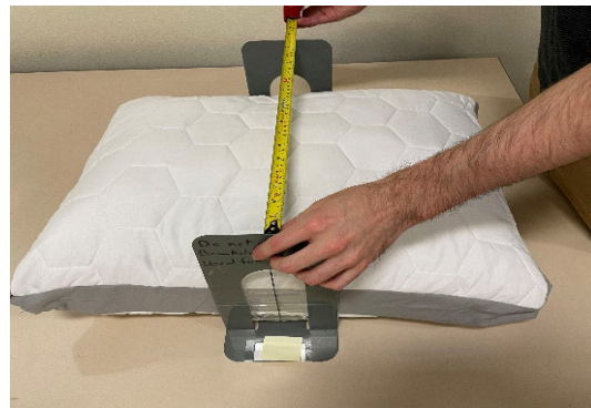
Figure 6: Width Measurement of Pillow with 90° Straightedges – Foam Pillows
