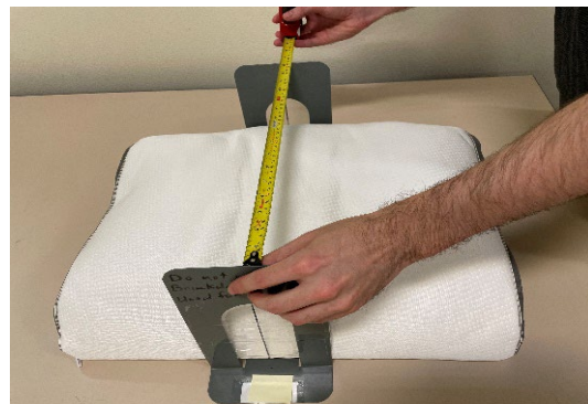
Figure 6: Width Measurement of Pillow with 90° Straightedges – Foam Pillows
