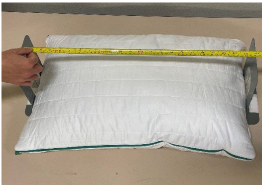
Figure 2: Length Measurement of Pillow with 90° Straightedges – Loose Fill Pillows
