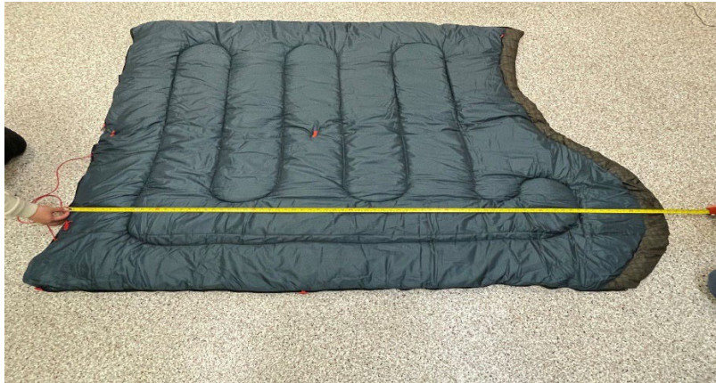
Figure 5: Measuring Length at Single Longest Point for Conventional Bag with Headrest / Attached Head Pillow
